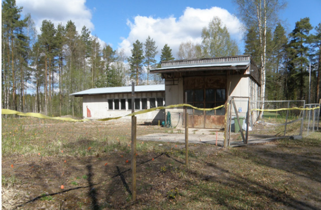
Phytoremediation is tested at the site. The seedlings of planted hybrid aspens have been marked with red flags. Photo: Niina Lallukka
