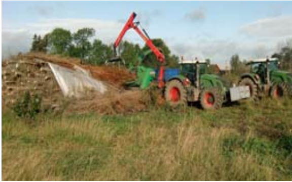
Feeding the chipper with the crane
